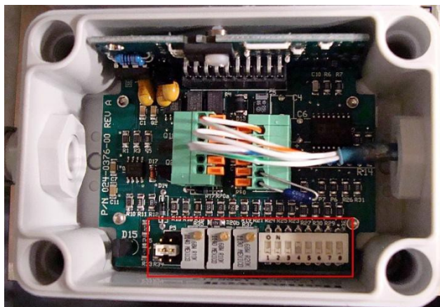
Figure 5-14: In-line Amplifier Interior View
