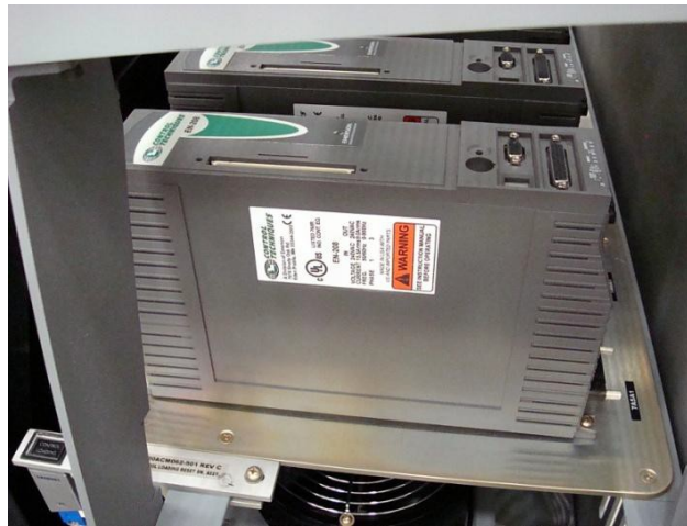
Figure 3-5. ECLS Servo Amps and Reset
