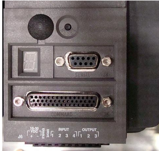
Figure 3-6. ECLS Servo Amp Front Panel
